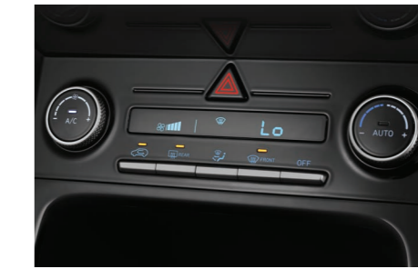
Full Automatic Temperature Controls
